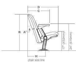
Three adjustable back angles (21°,18° and 15°) are provided to enhance spectator comfort and meet facility layout requirements.
