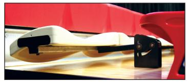
When folded down into the stored position, the contoured backrest sits above the deck. This protects both the deck and the backrest from marks and other damage.
